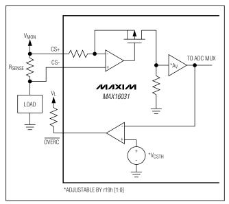
Figure 3. Current-Sense Block Diagram
