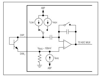
Figure 4. Remote Temperature Sensor Amplifier Circuitry
