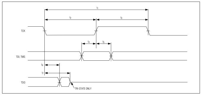
Figure 2. JTAG Interface Timing Diagram
