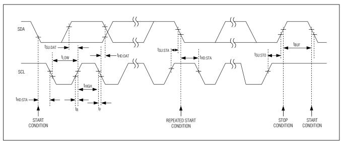
Figure 1. SMBus Interface Timing Diagram
