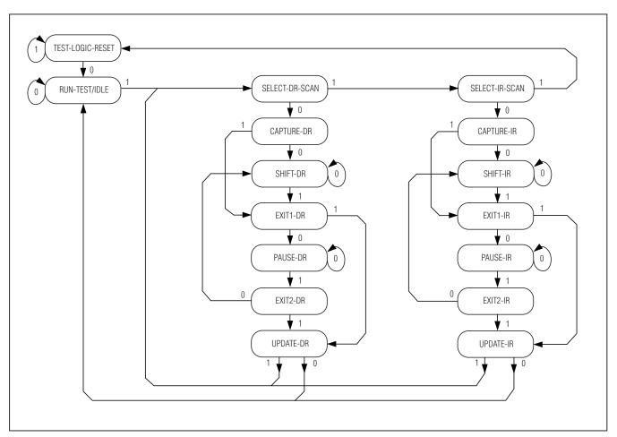
Figure 7. TAP Controller State Diagram
