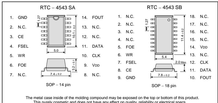
The metal case inside of the molding compound may be exposed on the top or bottom of this product. This purely cosmetic and does not have any effect on quality, reliability or electrical specs.
