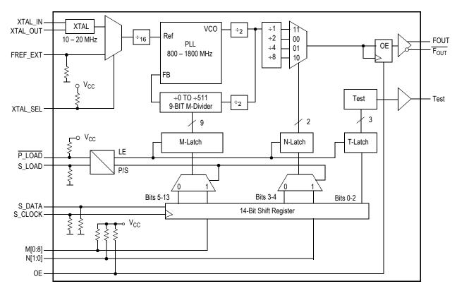
Figure 1. MPC9230 Logic Diagram
