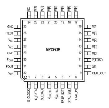
Figure 3. MPC9230 32-Lead Package Pinout (Top View)
