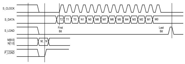
Figure 4. Serial Interface Timing Diagram
