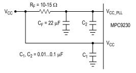
Figure 5. V<sub>CC\_PLL</sub> Power Supply Filter
