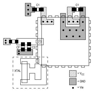
Figure 6. PCB Board Layout Recommendation for the PLCC28 Package
