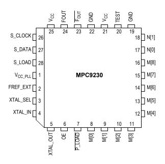
Figure 2. MPC9230 28-Lead PLCC Pinout (Top View)
