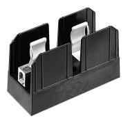
Catalog Symbol: J600 Series Ampere Rating: ½-600A Voltage Rating: 600V Withstand Rating: 200,000 RMS Sym. Amps For use with Class J Fuses (Bussmann LPJ, JKS) Agency Information: UL Listed, UL 512, Guide IZLT, File E14853 CSA Certified, C22.2 No. 39, Class 6225-01, File 47235 UL Flammability: 94VO Materials: Thermoplastic
