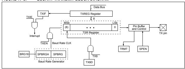
FIGURE 17-4: ASYNCHRONOUS TRANSMISSION
