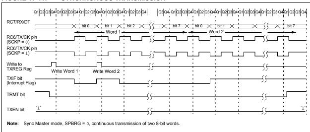
FIGURE 17-12: SYNCHRONOUS TRANSMISSION (THROUGH TXEN)
