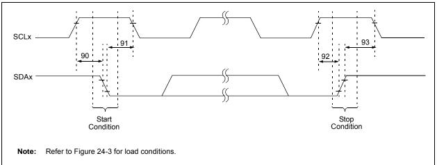
TABLE 24-20: MASTER SSP I<sup>2</sup>C™ BUS START/STOP BITS REQUIREMENTS
