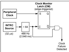
Clock failure is tested for on the falling edge of the sample clock. If a sample clock falling edge occurs while CM is still set, a clock failure has been detected (Figure 21-5). This causes the following:
