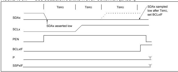
FIGURE 16-32: BUS COLLISION DURING A STOP CONDITION (CASE 2)
