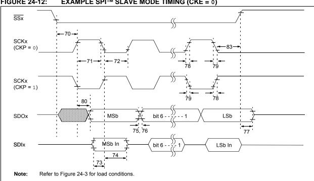
FIGURE 24-12: **EXAMPLE SPI™ SLAVE MODE TIMING (CKE = 0)**
