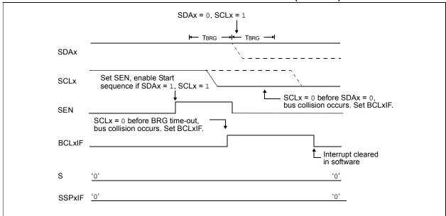
FIGURE 16-28: BRG RESET DUE TO SDAX ARBITRATION DURING START CONDITION
