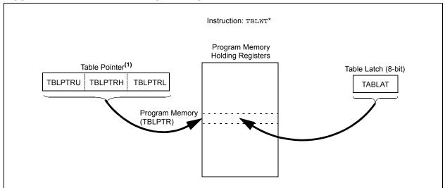
Note 1: Table Pointer actually points to one of 64 holding registers, the address of which is determined by TBLPTRL<5:0>. The process for physically writing data to the program memory array is discussed in Section 7.5 "Writing to Flash Program Memory".
