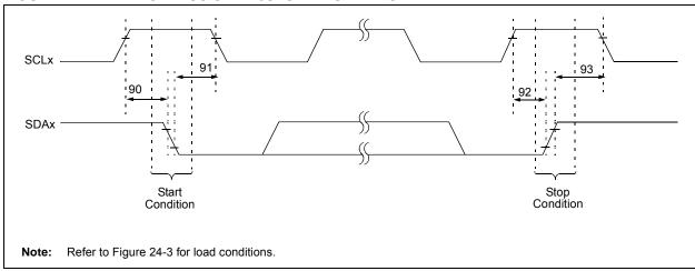
TABLE 24-18: I<sup>2</sup>C™ BUS START/STOP BITS REQUIREMENTS (SLAVE MODE)
