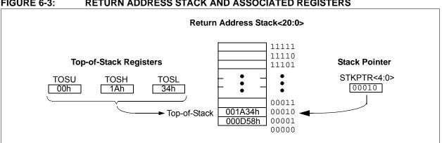
FIGURE 6-3: RETURN ADDRESS STACK AND ASSOCIATED REGISTERS
