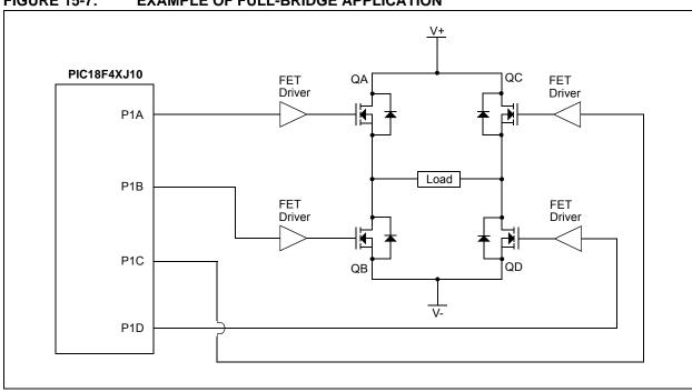
FIGURE 15-7: EXAMPLE OF FULL-BRIDGE APPLICATION
