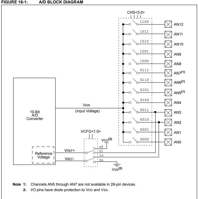
After the A/D module has been configured as desired, the selected channel must be acquired before the conversion is started. The analog input channels must have their corresponding TRIS bits selected as an input. To determine acquisition time, see **Section 18.1** "A/D Acquisition Requirements". After this acquisition time has elapsed, the A/D conversion can be started. An acquisition time can be programmed to occur between setting the GO/DONE bit and the actual start of the conversion.
