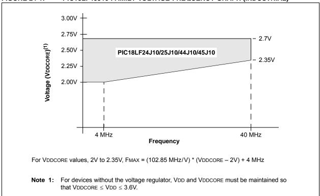
FIGURE 24-2: PIC18F45J10 FAMILY VOLTAGE-FREQUENCY GRAPH (INDUSTRIAL)
