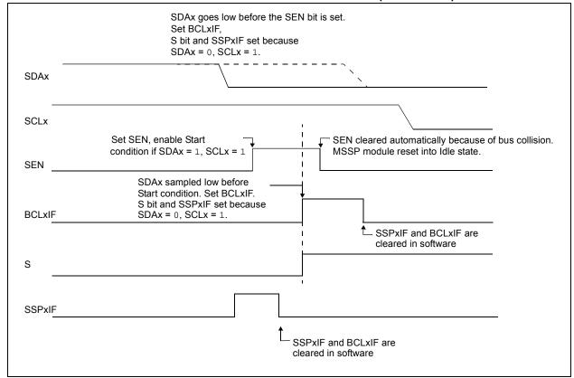
FIGURE 16-27: BUS COLLISION DURING START CONDITION (SCLx = 0)
