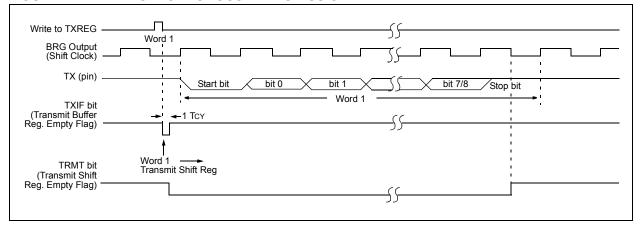
FIGURE 17-5: ASYNCHRONOUS TRANSMISSION (BACK TO BACK)
