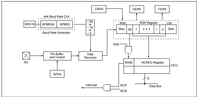
FIGURE 17-7: ASYNCHRONOUS RECEPTION
