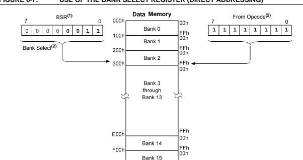
FIGURE 6-7: USE OF THE BANK SELECT REGISTER (DIRECT ADDRESSING)
