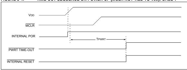
FIGURE 5-5: TIME-OUT SEQUENCE ON POWER-UP (MCLR NOT TIED TO VDD): CASE 2
