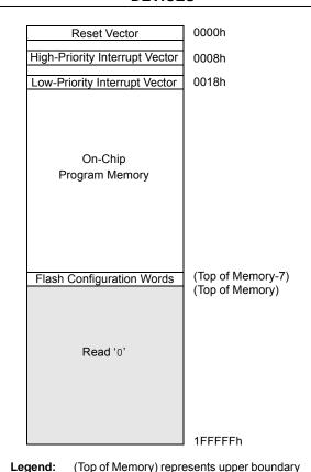
of on-chip program memory space (see Figure 6-1 for device-specific values). Shaded area represents unimplemented memory. Areas are not shown to scale.
