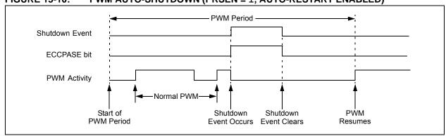
FIGURE 15-10: PWM AUTO-SHUTDOWN (PRSEN = 1, AUTO-RESTART ENABLED)
