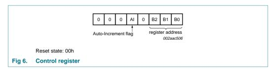
The lowest 3 bits are used as a pointer to determine which register will be accessed.
