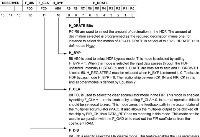
Bit FD0 is used to select the FIR disable mode. This feature enables the FIR parameters to be changed. This feature is selected by setting  $F\_DIS = 1$ . This mode terminates the current FIR cycle. While this feature is selected, the HDF continues to process data and write it into the FIR data RAM. When the FIR re-programming is completed, the FIR can be re-enabled either by clearing  $F\_DIS$ , or by asserting one of the start inputs, which automatically clears  $F\_DIS$ .
