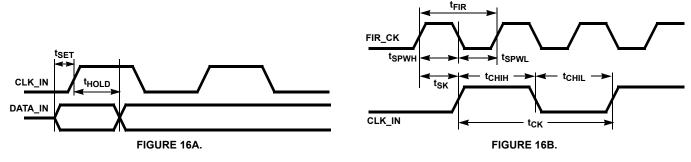
FIGURE 16. INPUT TIMING
