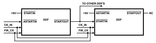
FIGURE 12. ASYNCHRONOUS START-UP
