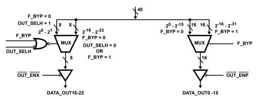
FIGURE 10. FIR OUTPUT FORMATTER
