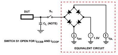
NOTE: Test head capacitance.
