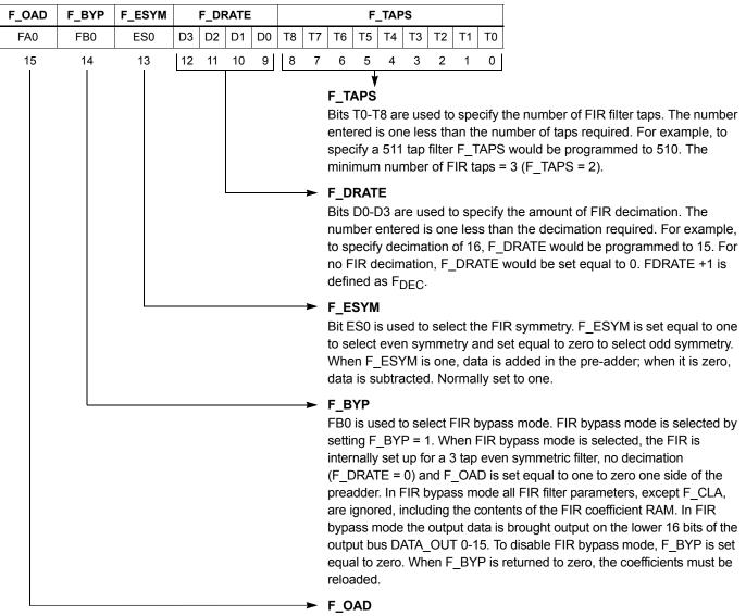
Bit FA0 is used to select the zero the preadder mode. This mode zeros one of the inputs to the pre-adder. Zero preadder mode is selected by setting F\_OAD equal to one. This feature is useful when implementing arbitrary phase filters or can be used to verify the filter coefficients. To disable the Zero Preadder mode F\_OAD is set equal to zero.
