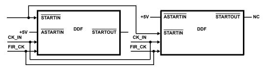
FIGURE 13. SYNCHRONOUS START-UP
