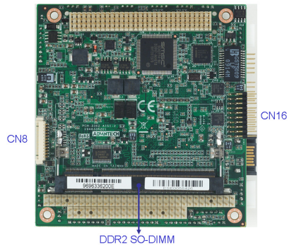
Figure 2: PCM-3362 Location Connectors & Jumpers (solder side)
