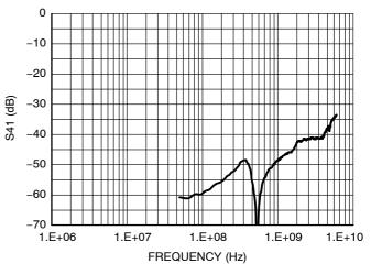
Figure 2. Analog Crosstalk Curve (S41 Measurement)
