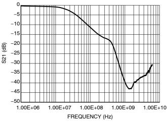
Figure 1. Typical Insertion Loss Characteristics (S21 Measurement)
