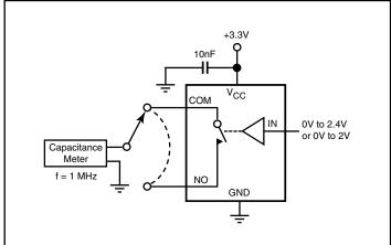
Figure 4. Channel On/Off Capacitance
