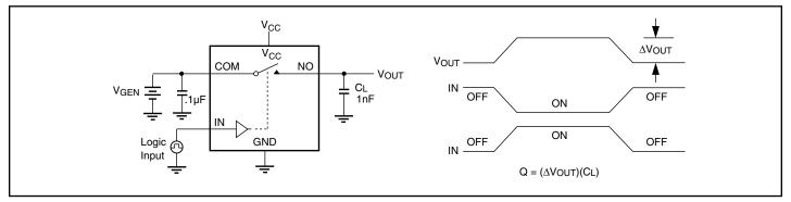
Figure 2. Charge Injection
