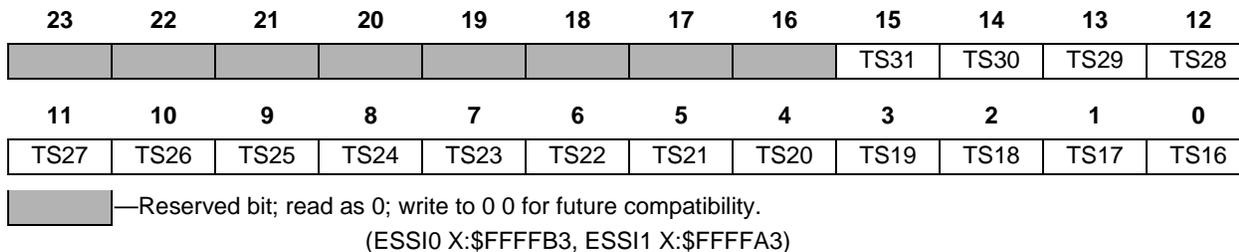
**Figure 7-15.** ESSI Transmit Slot Mask Register B (TSMB)
