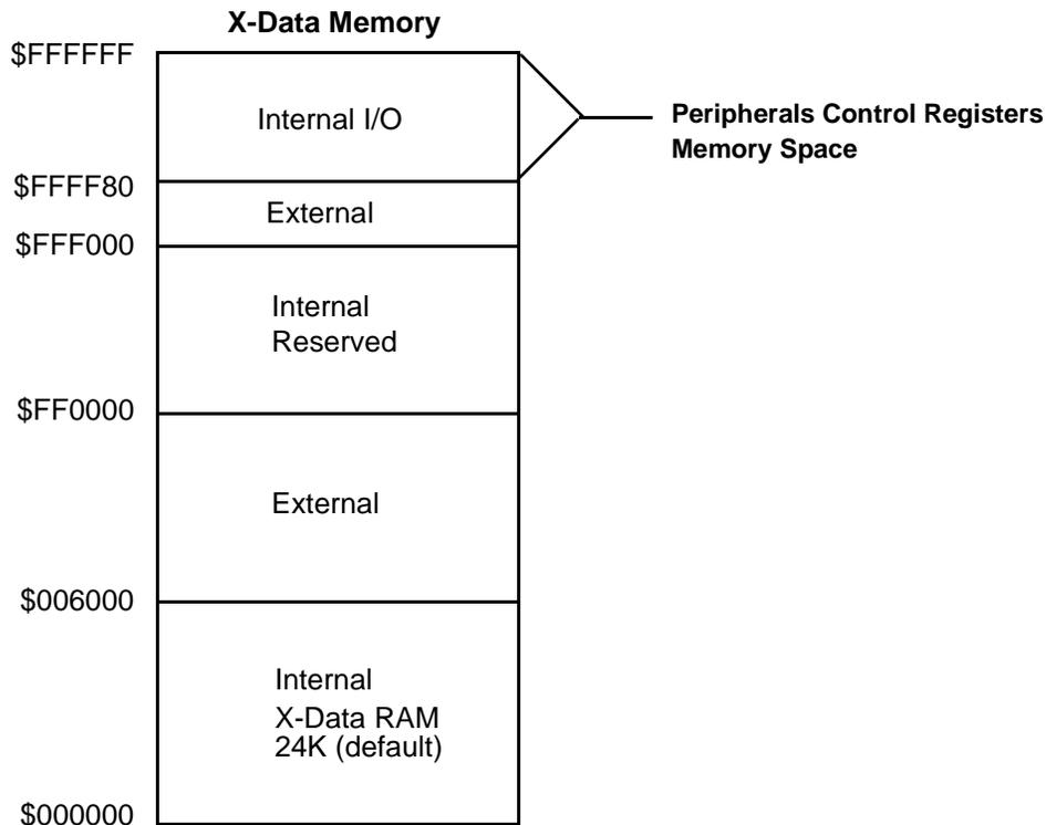
**Figure 5-1.** Memory Mapping of Peripherals Control Registers
