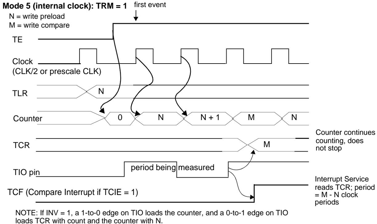
**Figure 9-13.** Period Measurement Mode, TRM = 1
