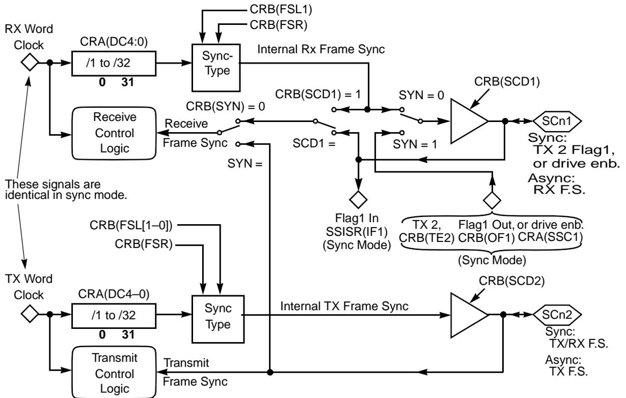
Figure 7-4. ESSI Frame Sync Generator Functional Block Diagram
