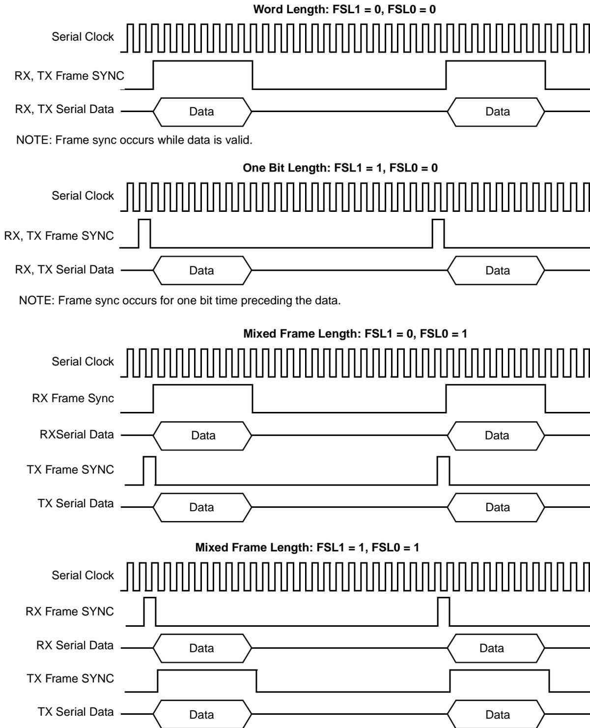
**Figure 7-6.** CRB FSL0 and FSL1 Bit Operation (FSR = 0)
