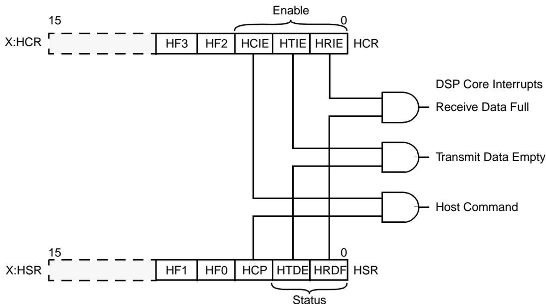
**Figure 6-2.** HI08 Core Interrupt Operation
