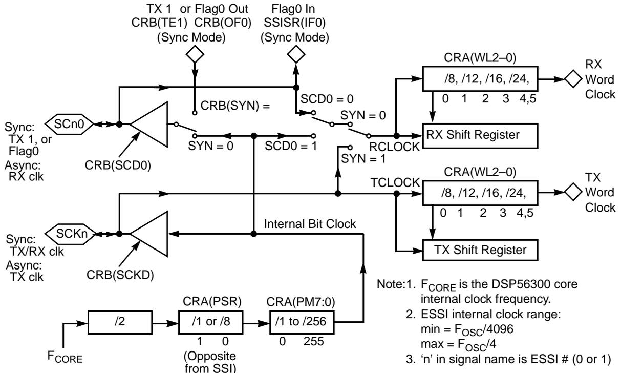
Figure 7-3. ESSI Clock Generator Functional Block Diagram
