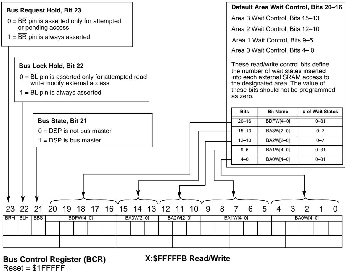
**Figure B-6. Bus Control Register (BCR)**
