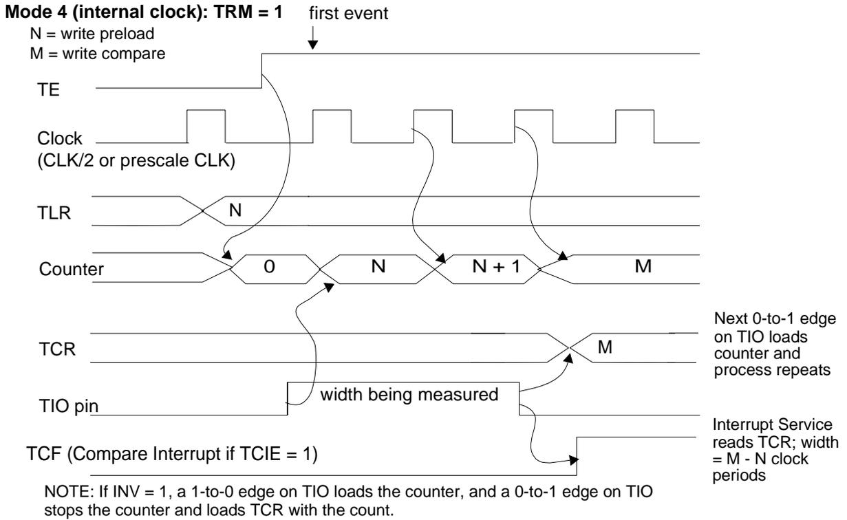
**Figure 9-11. Pulse Width Measurement Mode, TRM = 1**
