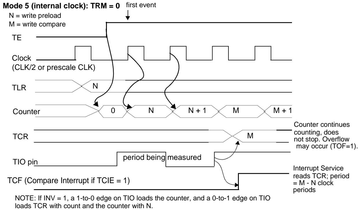
**Figure 9-14.** Period Measurement Mode, TRM = 0
