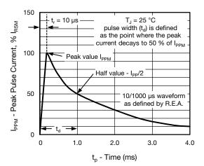
Fig. 3 - Pulse Waveform
