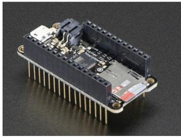
Finally, there's the "Stacking Header" option. This one is sort of the best-of-both-worlds. You get the ability to plug into a solderless breadboard *and* plug a featherwing on top. But its a little bulky
