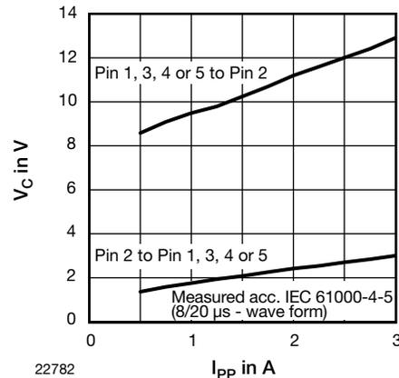
Fig. 6 - Typical Peak Clamping Voltage V<sub>C</sub> vs. Peak Pulse Current I<sub>PP</sub>
