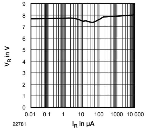
Fig. 5 - Typical Reverse Voltage V<sub>R</sub> vs. Reverse Current I<sub>R</sub>
