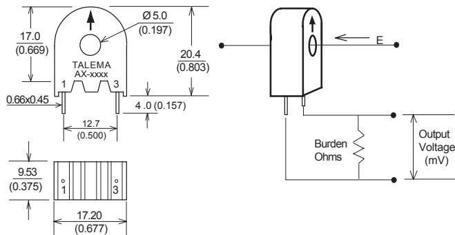
Dimensions are in mm. General Tolerance  $\pm 0.25\text{mm}$  unless specified.
