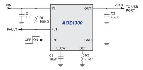
Figure 1. High Current USB Host
