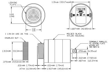
NOTE AF TERMINALS-032 BRASS TIN PLATED, TAPPED FOR #6-32 SCREW. TWO #6-32 NICKEL PLATED BRASS SCREWS INCLUED. WILL ACCEPT 1/4' QUICK CONNECT. NOTE B: MOUNTING- REMOVE BLACK PLASTIC NUT AND INSERT THREADED FRONT THROUGH 1.25' HOLE PUNCHED IN PANEL, IF DRIENTATION IS NEEDED, NOTE LOCKING FLATS ON DRAWING, SCREW NUT BACK ON. DO NOT DVERTIGHTEN.
