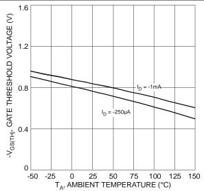
Fig. 17 Gate Threshold Variation vs. Ambient Temperature
