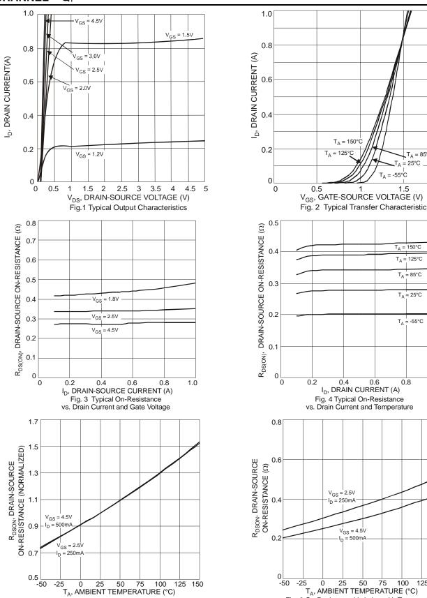
Fig. 5 On-Resistance Variation with Temperature
