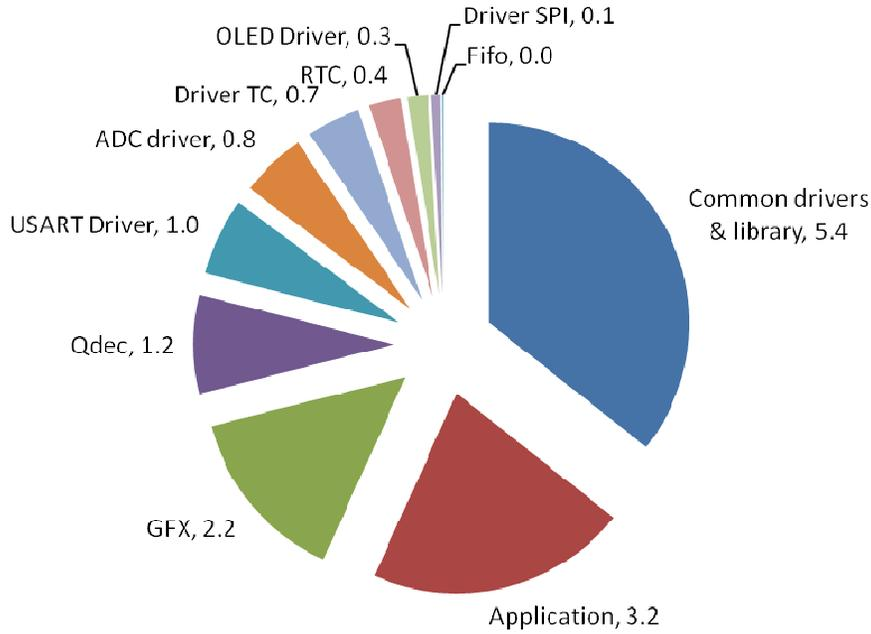
Figure 2-5. XMEGA-E5 Xplained demo RAM footprint (unit Byte).
