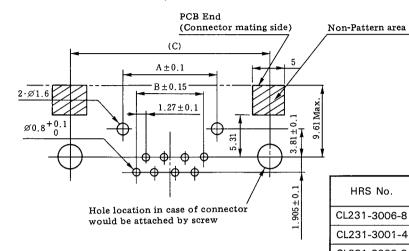
Unit:mm No. of Pin HRS No. С Part No. Α CL231-3006-8 9.96 6.35 23.96 3110-6S CL231-3001-4 8 3110-8S 12.5 8.39 26.5 CL231-3008-3 12 3110-12S 17.58 13.97 31.58 CL231-0018-0 3110-16S 22.66 19.05 36.66
