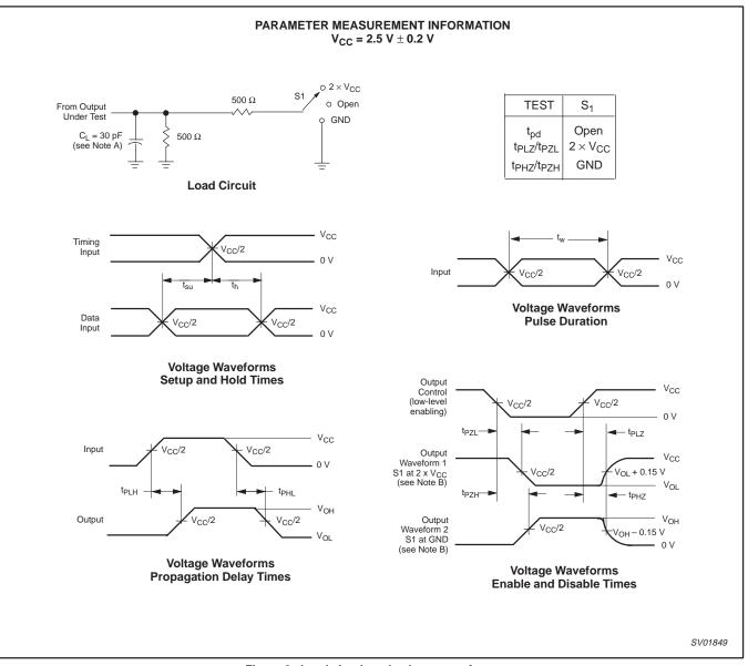
Figure 2. Load circuit and voltage waveforms
