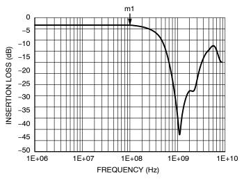
Figure 2. S21 Attenuation Simulation
