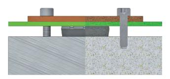
Figure 1: SMPD heat sink assembly
