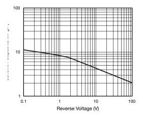
Fig. 4 - Typical Junction Capacitance
