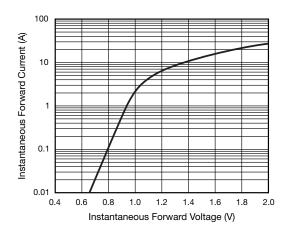
Fig. 2 - Typical Instantaneous Forward Characteristics Per Diode
