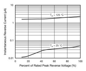
Fig. 3 - Typical Reverse Characteristics
