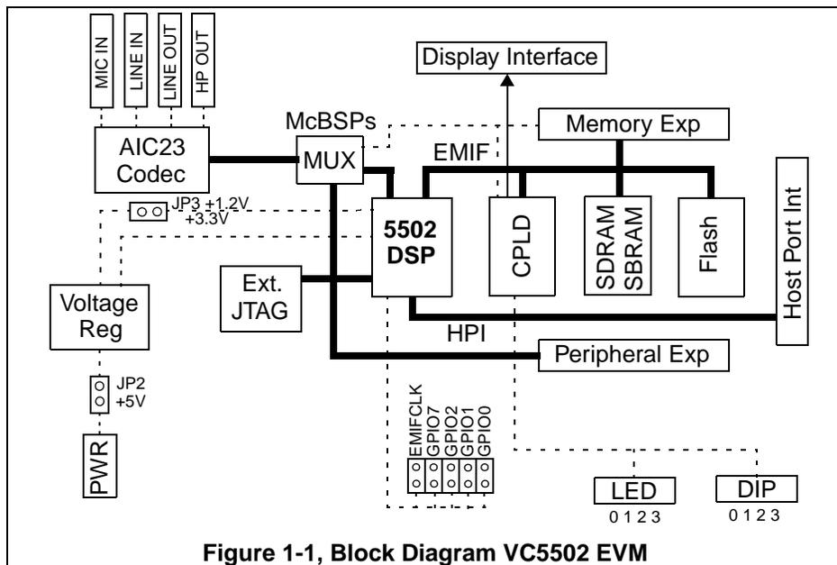
Figure 1-1, Block Diagram VC5502 EVM
