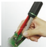
PCB Circuit Conductivity Test
