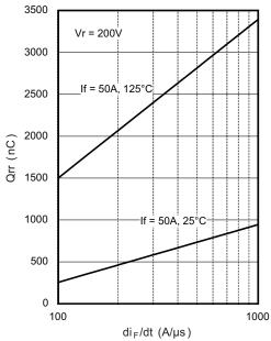
Fig. 7 - Typical Stored Charge vs. dl<sub>F</sub>/dt
