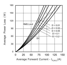
Fig. 5 - Forward Power Loss Characteristics (Per Leg)
