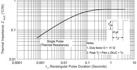
Fig. 3 - Maximum Thermal Impedance Z<sub>thJC</sub> Characteristics (Per Diode)
