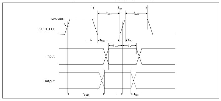
Table 50. SDIO Bus Timing<sup>1</sup> Parameters (High-Speed Mode)
