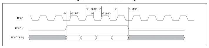
**Table 43. MII Receive Packet Timing Parameters**
