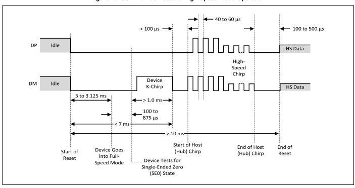
Figure 41 shows the USB 2.0 HS Mode transmit timing.
