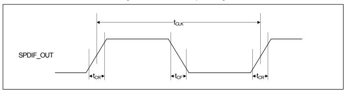
Table 54 provides the S/PDIF biphase mark code timing parameters (to be used in conjunction with Figure 34).
