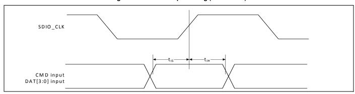
**Table 52. SDIO Bus Input Timing Parameters (SDR Modes)**
