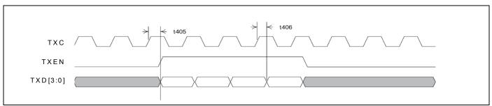
**Table 44. MII Transmit Packet Timing Parameters**
