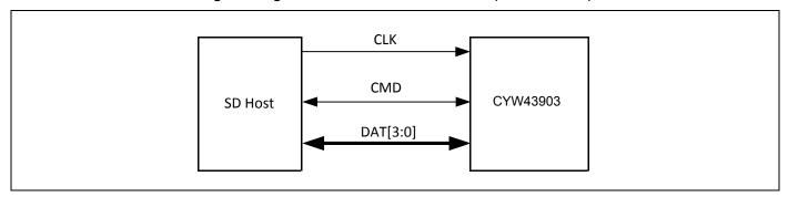
Figure 8. Signal Connections to an SDIO Host (SD 1-Bit Mode)
