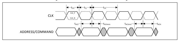
Figure 19. DDR3 DRAM Read Timing
