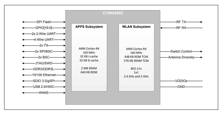
Figure 2. Block Diagram and I/O
