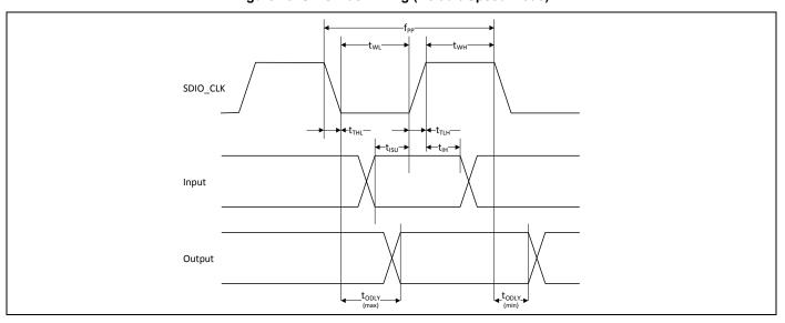
Table 49. SDIO Bus Timing<sup>1</sup> Parameters (Default-Speed Mode)
