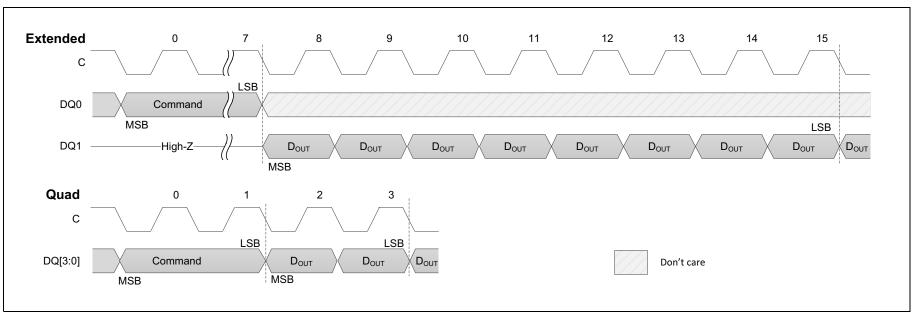
Figure 35. SPI Flash Read-Register Timing
