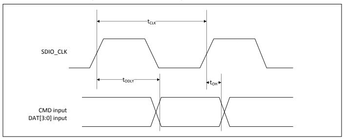
Table 53. SDIO Bus Output Timing Parameters (SDR Modes up to 50 MHz)
