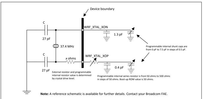
Figure 5. Recommended Oscillator Configuration
