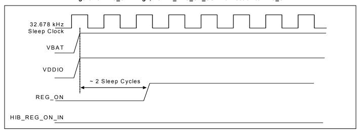
Figure 44. HIB\_REG\_ON\_IN = High, HIB\_REG\_ON\_OUT Connected to REG\_ON
