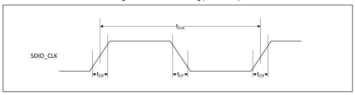
Table 51. SDIO Bus Clock Timing Parameters (SDR Modes)
