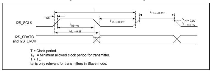
Figure 26 and Table 47 provide the I<sup>2</sup>S Slave mode receiver timing.
