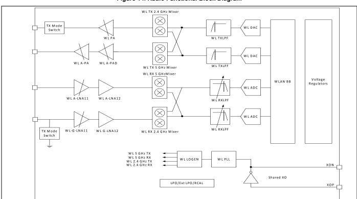
Figure 14. Radio Functional Block Diagram
