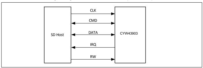
**Note:** Per Section 6 of the SDIO specification, pull-ups in the 10 k $\Omega$  to 100 k $\Omega$  range are required on the four data (DATA) lines and the command (CMD) line. This requirement must be met during all operating states either through the use of external pull-up resistors or through proper programming of the SDIO host's internal pull-ups
