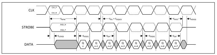
Figure 20. DDR3 DRAM Write Timing
