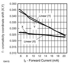
Figure 6. Chromaticity Coordinate Shift vs. Forward Current
