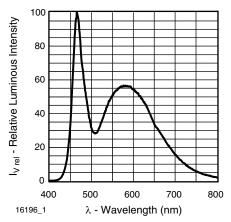
Figure 4. Relative Intensity vs. Wavelength
