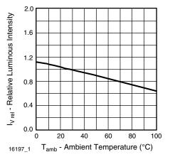
Figure 5. Rel. Luminous Intensity vs. Ambient Temperature
