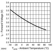
Figure 7. Forward Voltage vs. Ambient Temperature
