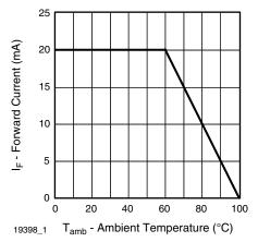
Figure 1. Forward Current vs. Ambient Temperature
