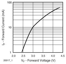
Figure 3. Forward Current vs. Forward Voltage
