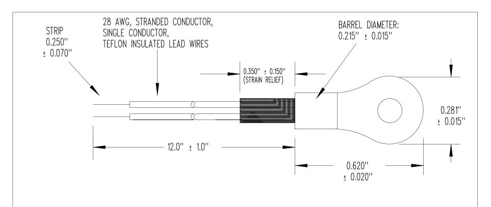
RTD ELEMENT RESISTANCE @ 0°C = 100  $\Omega$   $\pm$  0.24% RTD ELEMENT ACCURACY @ 0°C =  $\pm$  0.60°C TCR = 3,850ppm/°C RTD ELEMENT DIN 43760 ACCURACY CLASS = "C" MAXIMUM TEMPERATURE RATING = +150°C
