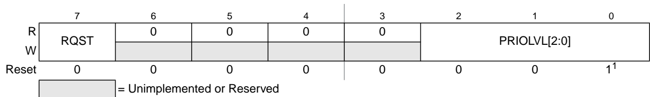
Figure 24-11. Interrupt Request Configuration Data Register 5 (INT_CFDATA5)
