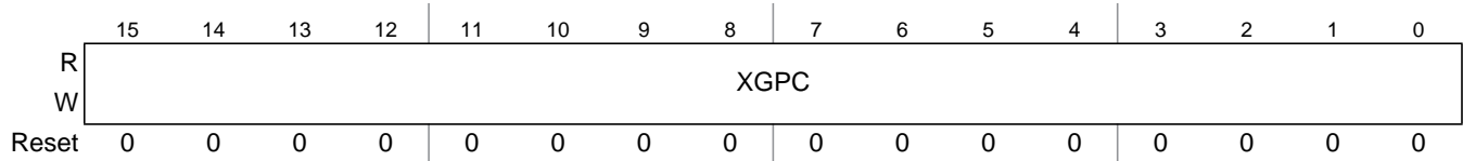
Figure 5-10. XGATE Program Counter Register (XGPC)
