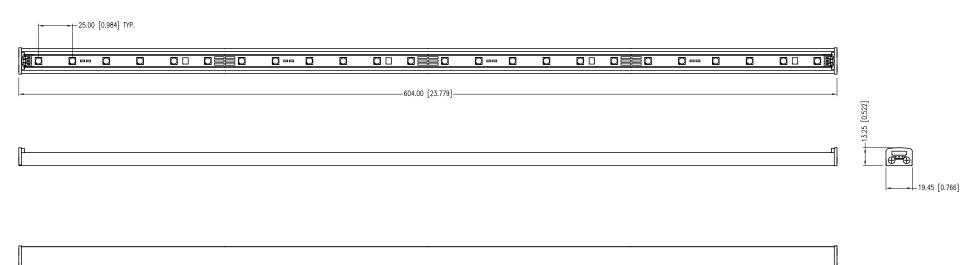
\*UNLESS OTHERWISE SPECIFIED TOLERANCES PER DECIMAL PRECISION ARE: X=±1 (±0.039), X.X=±0.5 (±0.020), X.XX=±0.25 (±0.010), X.XXX=±0.127 (±0.005). LEAD SIZE=±0.05 (±0.002), LEAD LENGTH=±0.75 (±0.030). MIN= +DECIMAL PRECISION ARX. = +0.00 | UNCONTROLLED DOCUMENT
