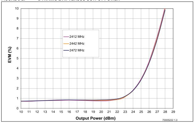
FIGURE 5-3: DYNAMIC EVM VERSUS OUTPUT POWER 802.11AC, MCS9-VHT40, 50% DUTY CYCLE
