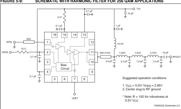
FIGURE 5-9: SCHEMATIC WITH HARMONIC FILTER FOR 256 QAM APPLICATIONS
