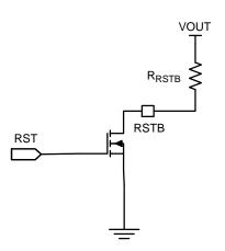
Figure 10. Reset with Adjustable Delay on a Single Pin
