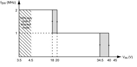
Figure 9. NCV890430 Worst-Case Switching Frequency Profile vs. Input Voltage
