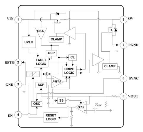
Figure 2. Simplified Block Diagram
