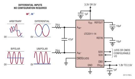
The LTC<sup>®</sup>2311-14 is a low noise, high speed 14-bit + sign successive approximation register (SAR) ADC with differential inputs and wide input common mode range. Operating from a single 3.3V or 5V supply, the LTC2311-14 has an  $8V_{P-P}$  differential input range, making it ideal for applications which require a wide dynamic range with high common mode rejection. The LTC2311-14 achieves ±0.75LSB INL typical, no missing codes at 14 bits and 80dB SNR typical.
