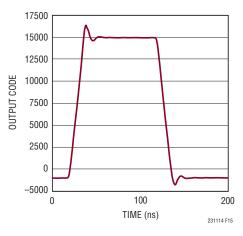
Figure 15. Transient Response of the LTC2311-14
