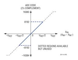
Figure 5. Pseudo-Differential Bipolar Transfer Function
