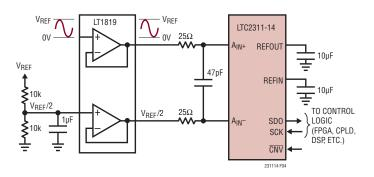
Figure 4. Pseudo-Differential Bipolar Application Circuit
