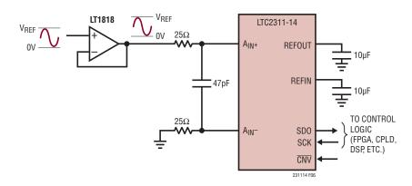
Figure 6. Pseudo-Differential Unipolar Application Circuit
