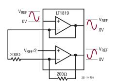
Figure 8. Single-Ended to Differential Driver
