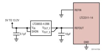
Figure 13b. LTC2311-14 with an External REFOUT Voltage
