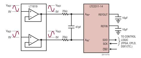
Figure 10. Fully-Differential Application Circuit
