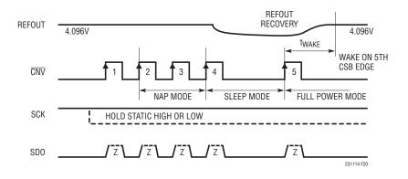
Figure 20. LVDS and CMOS Mode SLEEP and WAKE Using  $\overline{\text{CNV}}$
