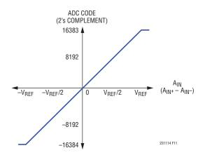
Figure 11. Fully-Differential Transfer Function
