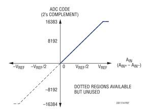
Figure 7. Pseudo-Differential Unipolar Transfer Function
