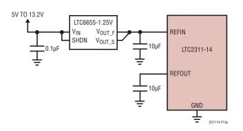
Figure 13a. LTC2311-14 with an External REFIN Voltage
