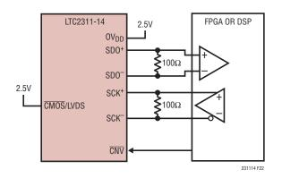
Figure 22. LTC2311-14 Using the LVDS Interface
