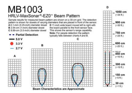
The different HRLV models have different beam width patterns, check this image for a comparison of all the HRLV model beam patterns. If you don't need high sensitivity, or want a longer range, check out the LV models – They are meant for up to 6.5 meter distances
