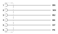
Contact assignment of M8 socket
