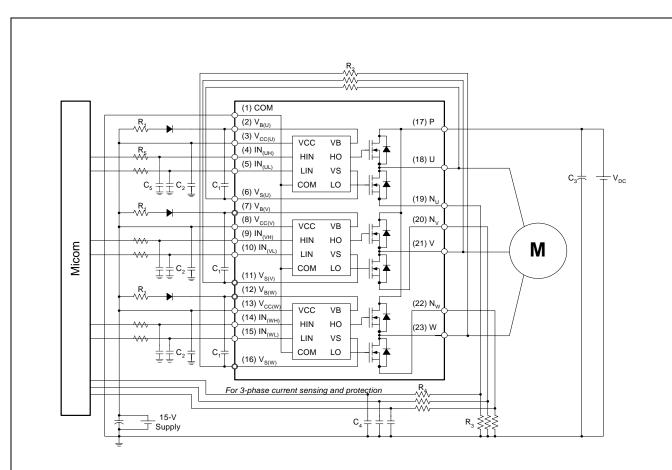
Figure 8. Example of Application Circuit
