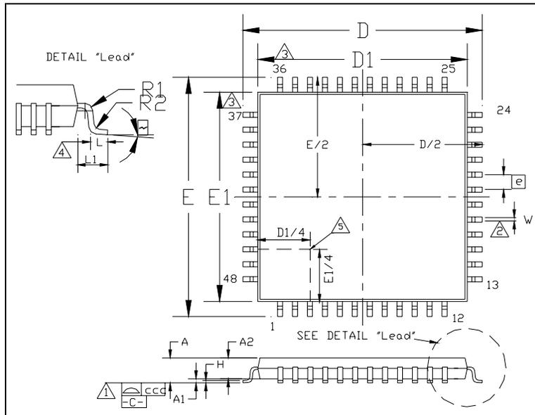
Figure 2 - COM20022I 48 Pin TQFP Package Outline
