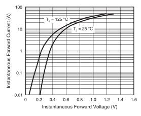
Fig. 3 - Typical Instantaneous Forward Characteristics
