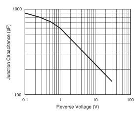
Fig. 5 - Typical Junction Capacitance
