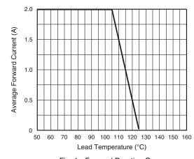
Fig. 1 - Forward Derating Curve
