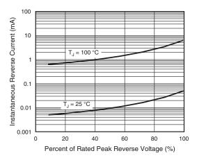
Fig. 4 - Typical Reverse Current Characteristics
