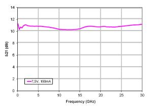
Typical IC performance measured on-wafer
