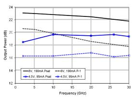
Typical IC performance measured on-wafer
