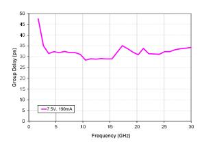
Typical IC performance measured on-wafer
