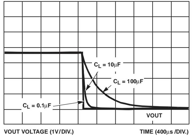
FIGURE 9. FAST TURN-OFF vs  $C_{LOAD}$
