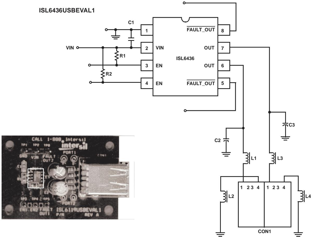
FIGURE 20. ISL6436USBEVAL BOARD
