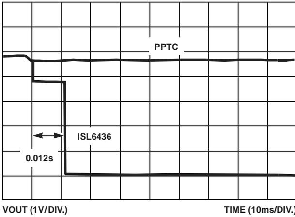
FIGURE 14. ISL6436 vs PPTC PLUGGED ONTO 1.5A LOAD
