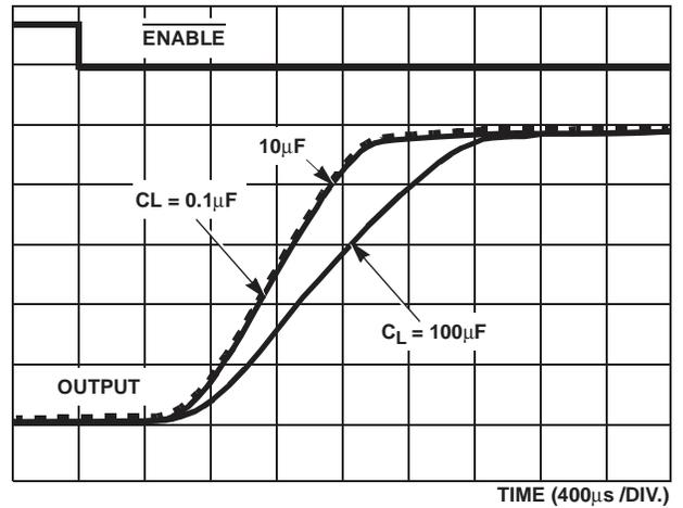
FIGURE 3. VOUT SOFT START vs  $C_{LOAD}$ ,  $R_I = 10\Omega$
