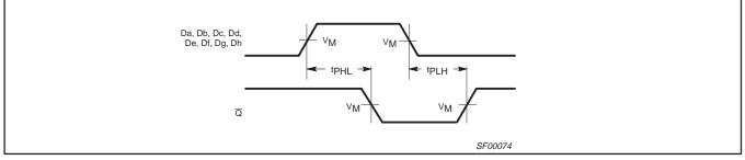
Waveform 1. Propagation Delay for Inverting Outputs
