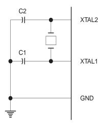
Note: C1, C2 = 30 pF  $\pm$ 10 pF for Crystals = 40 pF  $\pm$ 10 pF for Ceramic Resonators
