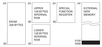
With EXTRAM = 0, the ERAM is indirectly addressed, using the MOVX instruction in combination with any of the registers R0, R1 of the selected bank or DPTR. An access to ERAM will not affect ports P0, P2, P3.6  $(\overline{WR})$ , and P3.7  $(\overline{RD})$ . For example, with EXTRAM = 0,
