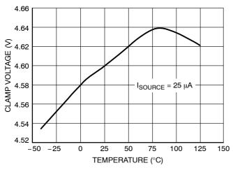
Figure 13. Control Input Upper Window Clamp
