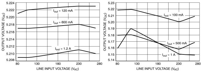
Figure 30. Converter Line Regulation
