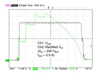
Figure 39. Charger On/Off Line Transient Response
