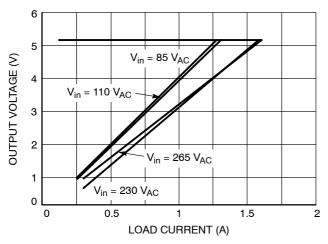
Figure 32. Converter Load Regulation
