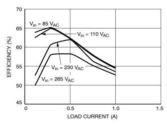
Figure 37. Charger Efficiency
