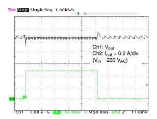
Figure 35. Charger Load Transient Response
