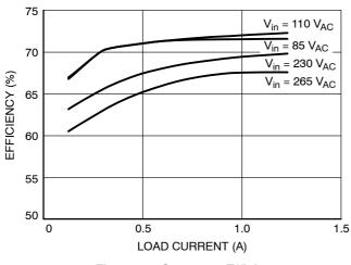
Figure 36. Converter Efficiency
