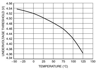
Figure 19. Undervoltage Lockout Threshold versus Temperature
