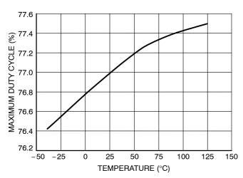
Figure 9. Maximum Duty Cycle versus Temperature
