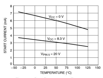
Figure 20. Start Current versus Temperature
