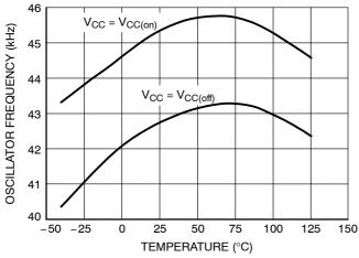
Figure 5. Oscillator Frequency
