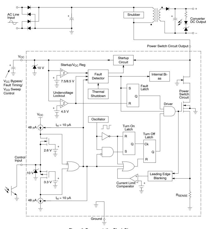
Figure 2. Representative Block Diagram
