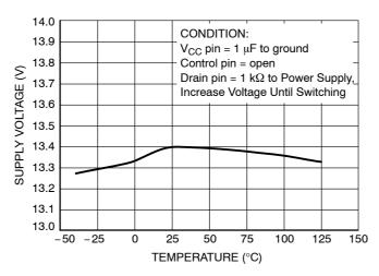
Figure 27. Supply Voltage versus Temperature
