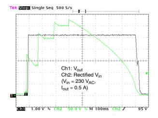
Figure 38. Converter On/Off Line Transient Response
