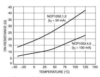
Figure 14. On Resistance versus Temperature
