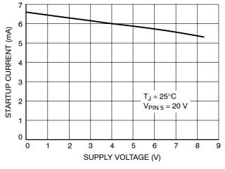
Figure 21. Startup Current versus Supply Voltage
