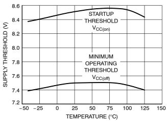
Figure 18. Supply Voltage Thresholds versus Temperature
