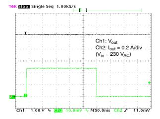
Figure 34. Converter Load Transient Response
