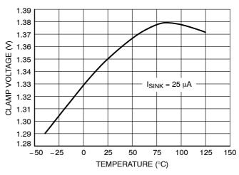
Figure 12. Control Input Lower Window Clamp
