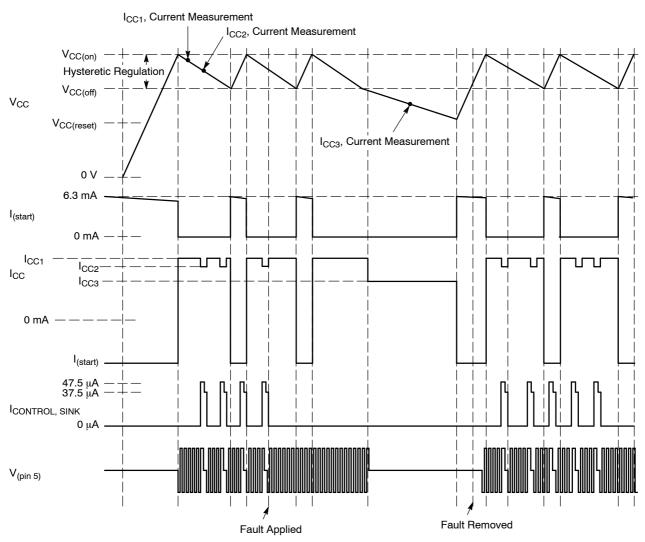
Figure 4. Non-Latching Fault Condition Timing Diagram
