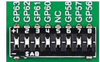
Figure 6-3: Tri-state DIP switch on PORT00-07
