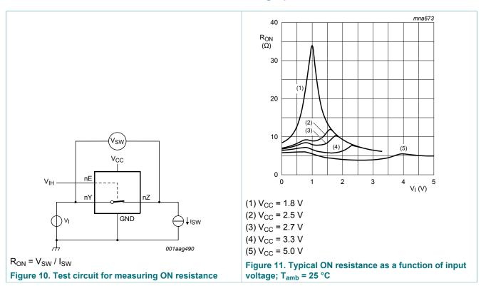
Typical values are measured at  $T_{amb}$  = 25 °C and nominal  $V_{CC}$ . Flatness is defined as the difference between the maximum and minimum value of ON resistance measured at identical  $V_{CC}$  and temperature.
