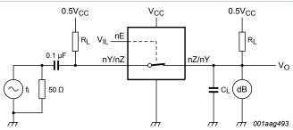
Adjust fi voltage to obtain 0 dBm level at input.
