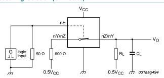
Figure 23. Test circuit for measuring crosstalk voltage (between digital inputs and switch)
