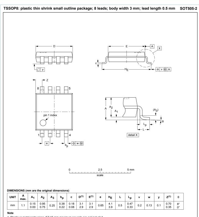
1. Plastic or metal protrusions of 0.15 mm maximum per side are not included.
