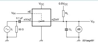
$\label{eq:definition} Adjust \ f_i \ voltage \ to \ obtain \ 0 \ dBm \ level \ at \ output. \ Increase \ f_i \ frequency \ until \ dB \ meter \ reads \ -3 \ dB.$
