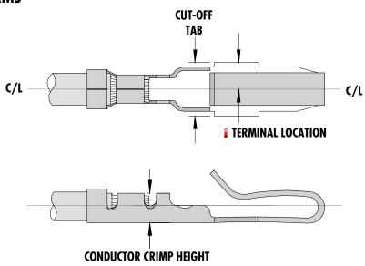
♣ Terminal is to be centrally located between the two (2) cut-off tab edges by one half of the total cut-off tab tolerance. This illustration is a generic terminal representation and not an exact image of any terminal listed in the scope.
