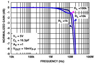
FIGURE 5. GAIN vs FREQUENCY vs RL
