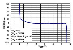
FIGURE 19. INPUT OFFSET CURRENT vs COMMON-MODE INPUT VOLTAGE
