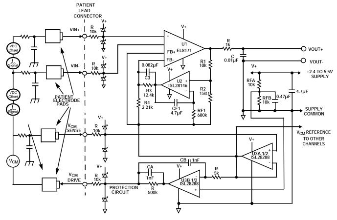
FIGURE 38. ECG/EEG AMPLIFIER
