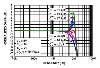
FIGURE 8. GAIN vs FREQUENCY vs CL
