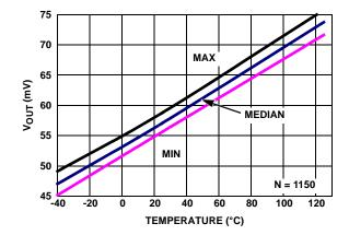
FIGURE 35.  $V_{OUT}$  LOW vs TEMPERATURE  $V_+$ ,  $V_-$  =  $\pm 2.5V$ ,  $R_L$  = 1k
