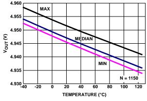
FIGURE 34.  $V_{OUT}$  HIGH vs TEMPERATURE  $V_+$ ,  $V_- = \pm 2.5V$ ,  $R_1 = 1k$
