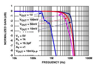
FIGURE 2. GAIN vs FREQUENCY vs  $V_{OUT}$ ,  $R_L = 1k$
