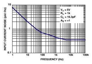
FIGURE 13. INPUT CURRENT NOISE DENSITY vs FREQUENCY
