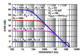
FIGURE 6. FREQUENCY RESPONSE vs CLOSED LOOP GAIN
