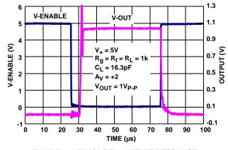
FIGURE 17. ENABLE TO OUTPUT RESPONSE
