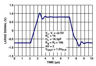
FIGURE 15. LARGE SIGNAL STEP RESPONSE
