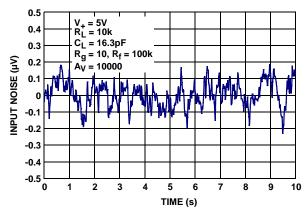
FIGURE 14. INPUT VOLTAGE NOISE 0.1Hz to 10Hz
