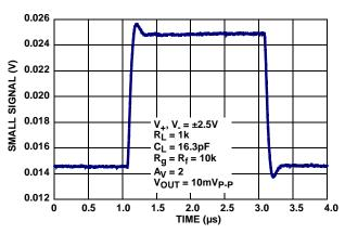
FIGURE 16. SMALL SIGNAL STEP RESPONSE
