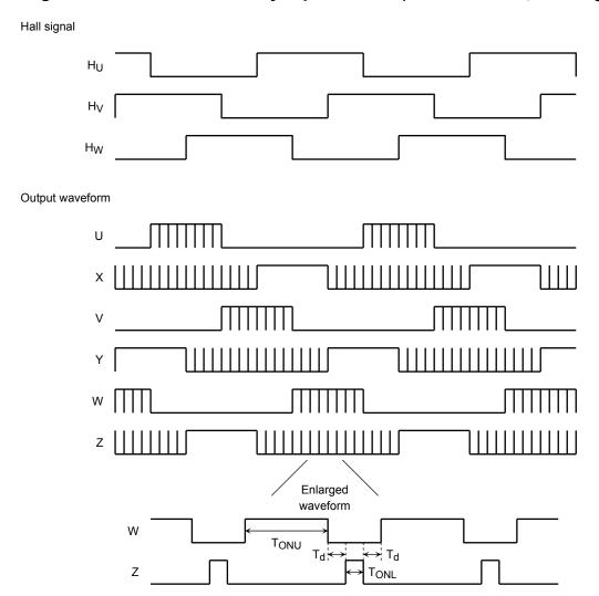
To stabilize the bootstrap voltage, the lower outputs  $(X,\,Y,\,\text{and}\,Z)$  are always turned on at the carrier cycle even during off time. At that time, the upper outputs  $(U,\,V,\,\text{and}\,W)$  are assigned dead time and turned off at the timing when the lower outputs are turned on.  $(T_d\,\text{varies}\,\text{with}\,\text{input}\,V_e.)$
