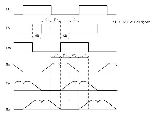
In the above diagram, the modulation waveform (1)' data moves forward by the 1/32 time width of the time (1) from HU:  $\downarrow$  to HW:  $\uparrow$  Similarly, data (2)' moves forward by the 1/32 time width of the time (2) from HW:  $\uparrow$  to HV:  $\downarrow$ .
